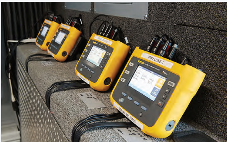
Multiple three-phase power monitors set up to ensure continued flow during a professional football league game
