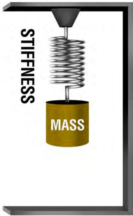
Figure 1: A spring-mass harmonic isolator best describes Hooke's law
