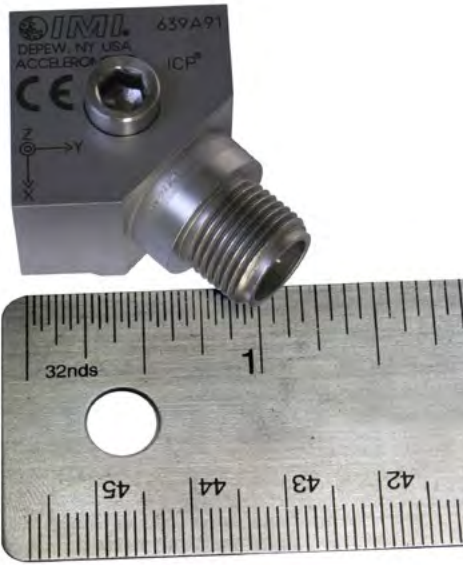
Figure 3: A triaxial accelerometer with a footprint less than one inch square and a 13kHz frequency response on all three axes
